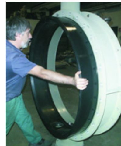
ND 60" NP 10 Flanged, fabricated body, replaceable seat
