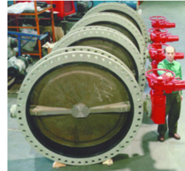
ND 60" AWWA Cl.D Flanged, replaceable seat POWER PLANT
